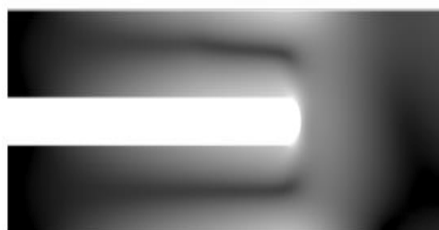
Fig. 4. Simulation of the volume strain of the quartz tuning fork.
